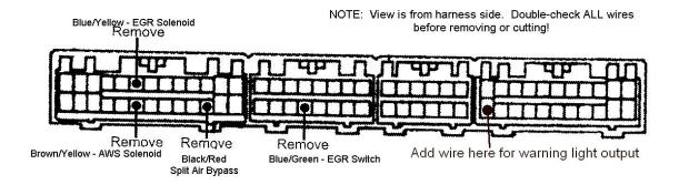
Install your additional wire into that spot, and part 1 is done. The wire will just pop into that spot, just install until it clicks into place. The connector is keyed so it will only install one way.
