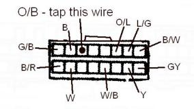
So, strip a bit of that orange/black wire back, solder a decent length of wire (probably 2 feet or so) to the stripped back portion, and wrap with tape. Attach the other end to the wire you added to the ECU for pin 1V. I used a quick-disconnect on the ECU side so I can easily disconnect the wire if I ever need to put the stock ECU back in or something.
