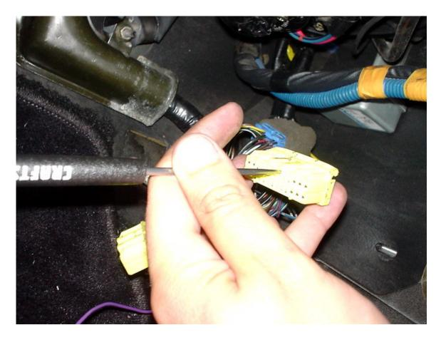
Lift up on the tang, and pull the wire on the other side. If you get it just right, the pin will slide out nice and easy. It's easier done than said, actually. This is also how you would remove a wire from a junkyard connector, or get an extra wire from your harness to move to the right position.
