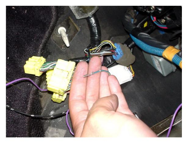
Time to install the wire. It goes into terminal 1V on the ECU. On the US harness, this spot on the harness will not have a wire on it. Here's a diagram showing the location –
