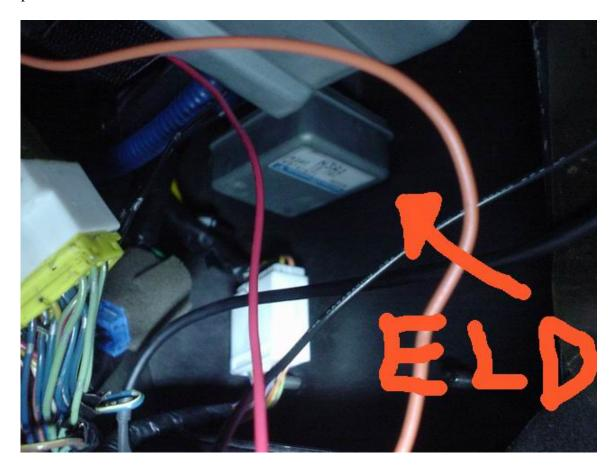
The wire on the harness is an ORANGE/BLACK STRIPE wire. Here's a diagram of the ELD connector that I hand-made –
